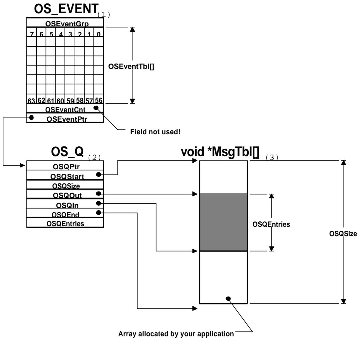
**Figure 6-8, Data structures used in a message queue.**
