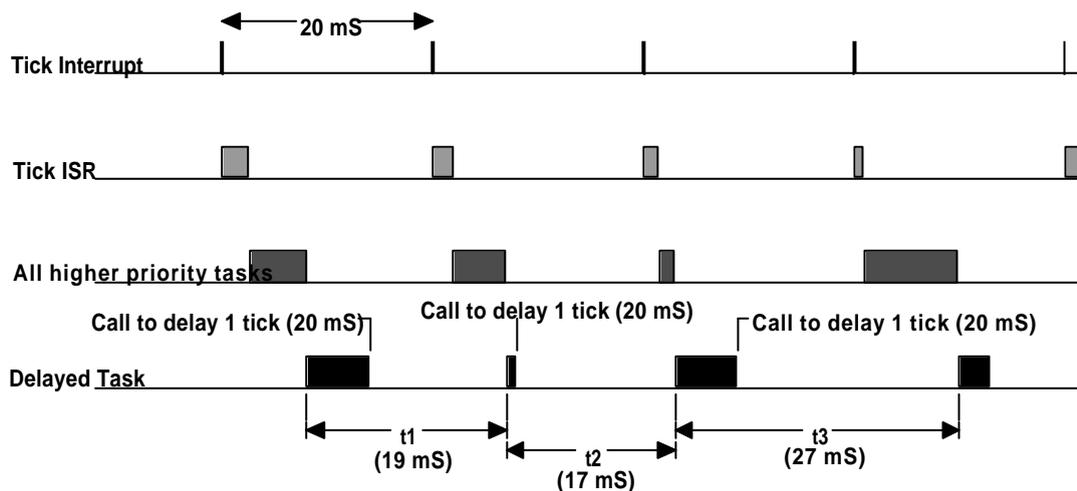
**Figure 2-24, Delaying a task for 1 tick (case #1).**
