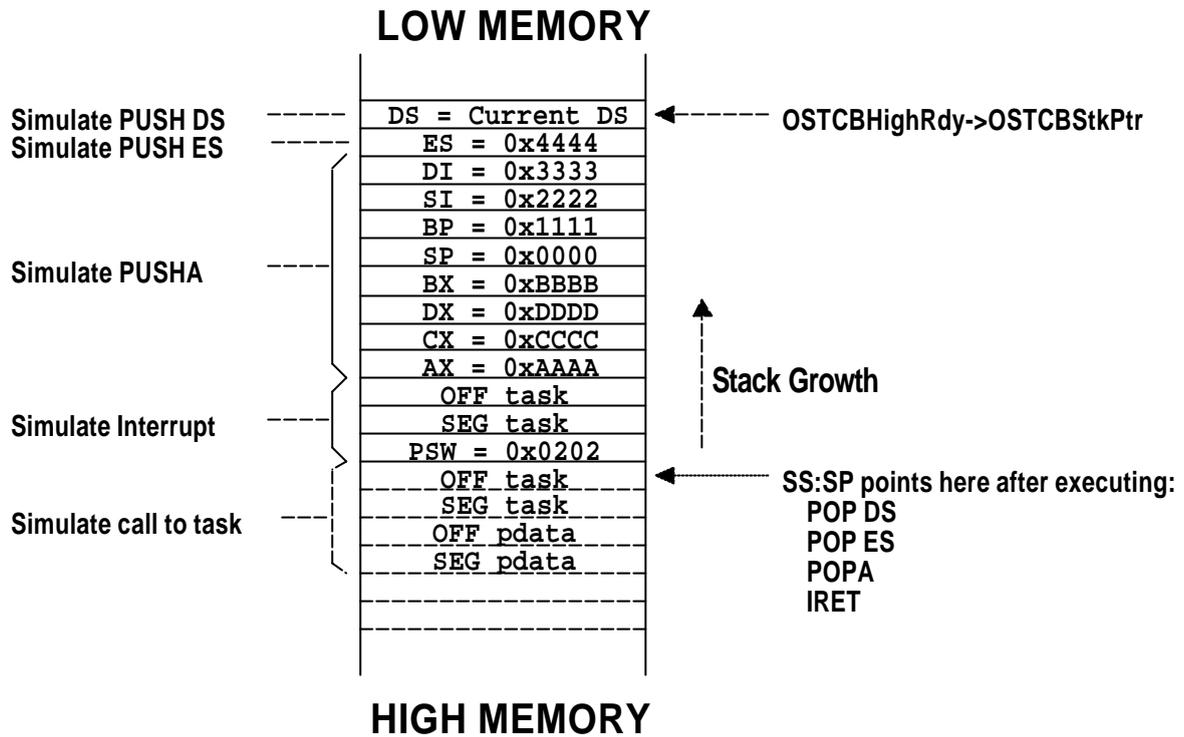
**Figure 9-3, 80x86 Stack frame when task is created**
