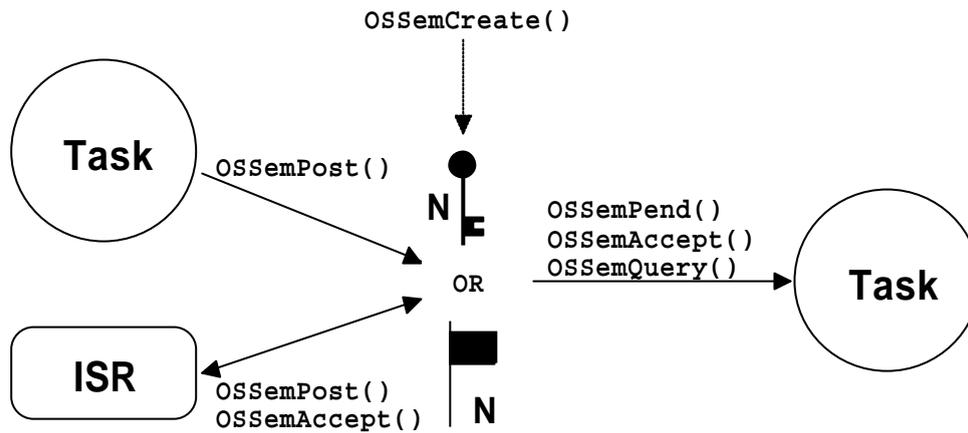
**Figure 6-5, Relationship between tasks, ISRs and a semaphore.**
