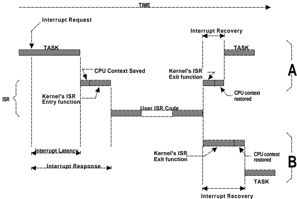
**Figure 2-21, Interrupt latency, response, and recovery (Preemptive kernel)**
