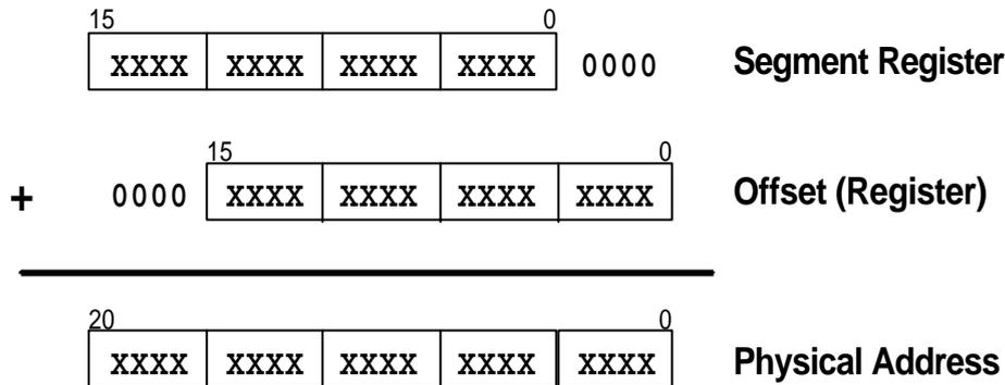
**Figure 9-2, Addressing with a Segment and an Offset**
