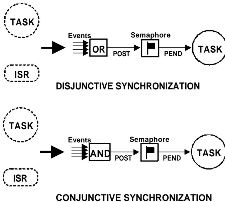
**Figure 2-14, Disjunctive and conjunctive synchronization.**
