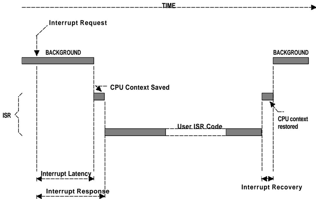
**Figure 2-19, Interrupt latency, response, and recovery (Foreground/Background)**
