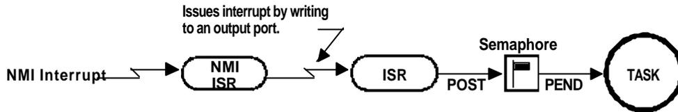
**Figure 2-23, Signaling a task from a non-maskable interrupt.**
