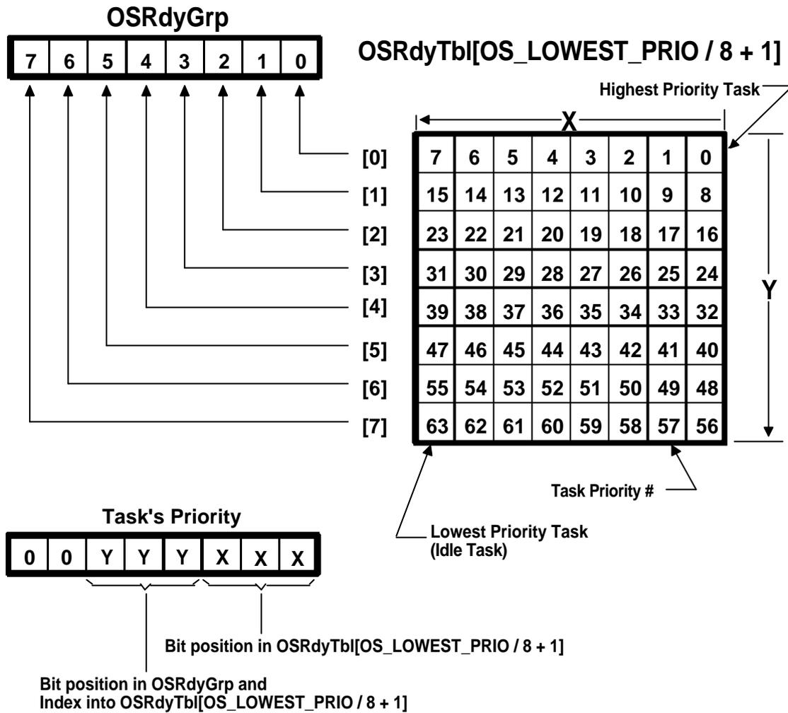
**Figure 3-3,  $\mu\text{C/OS-II}$ 's Ready List**
