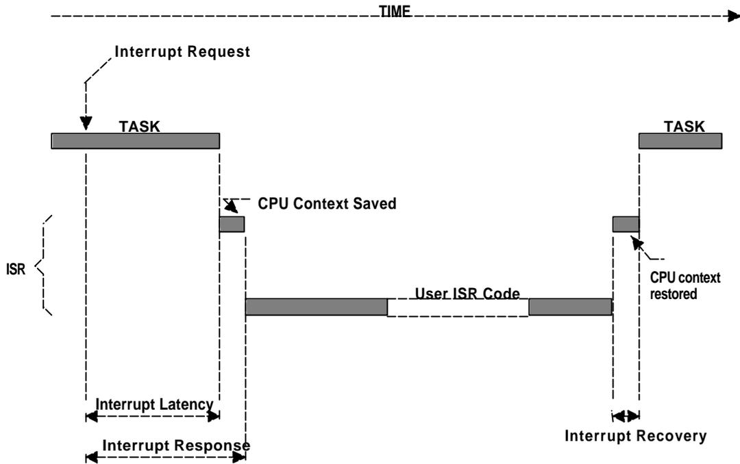
**Figure 2-20, Interrupt latency, response, and recovery
