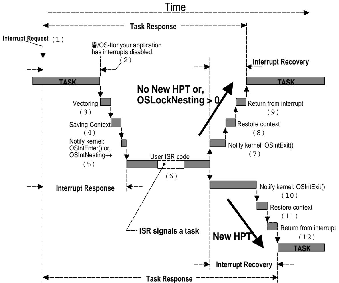
**Figure 3-5, Servicing an interrupt**
