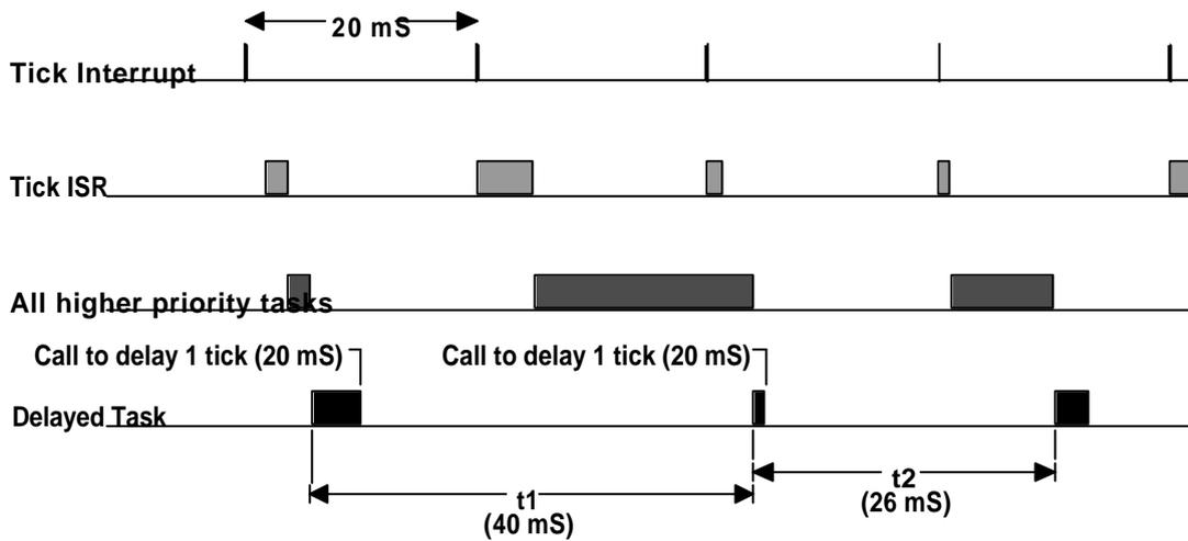
**Figure 2-26, Delaying a task for 1 tick (case #3).**
