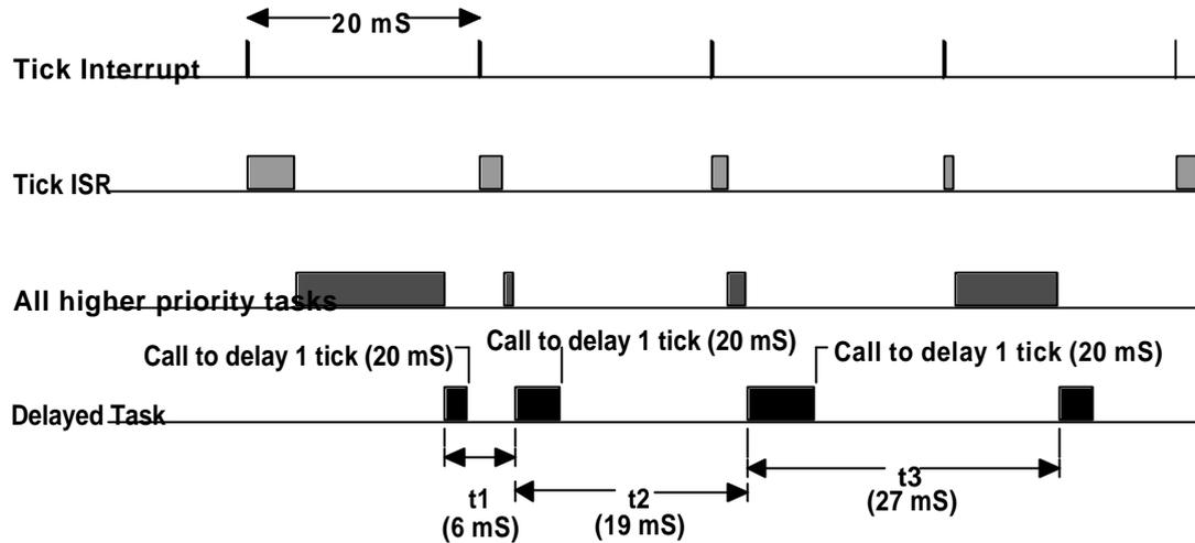
**Figure 2-25, Delaying a task for 1 tick (case #2).**
