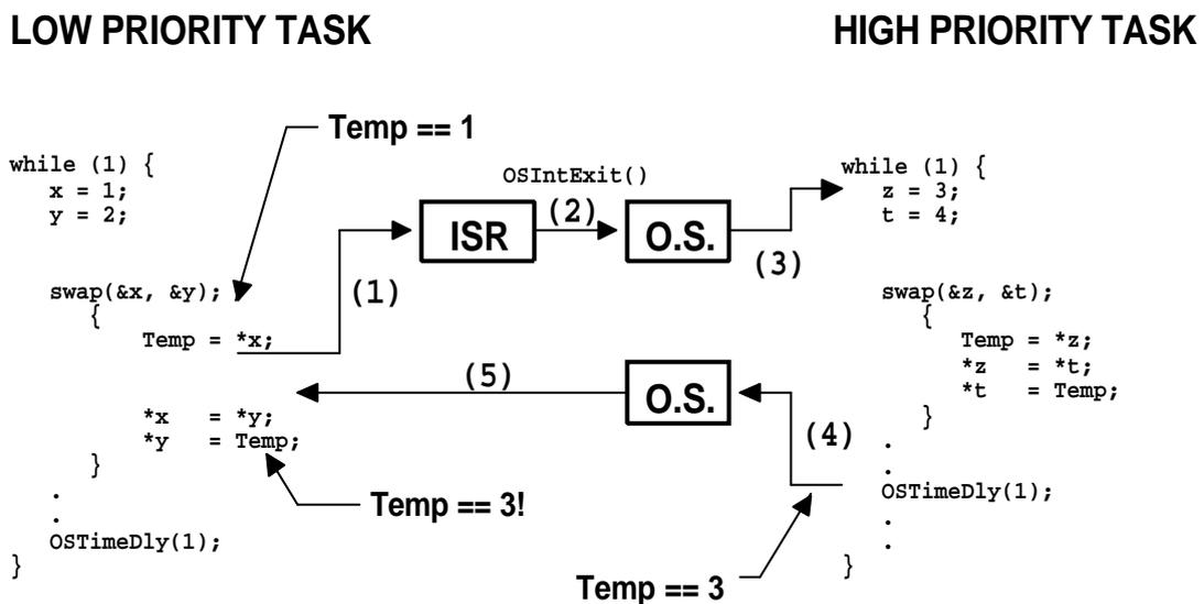
Figure 2-6, Non-reentrant function.
