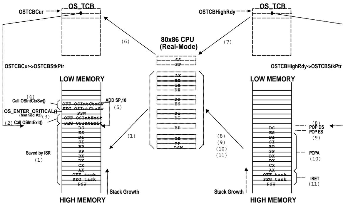
**Figure 9-5, 80x86 Stack frames during an interrupt level context switch**
