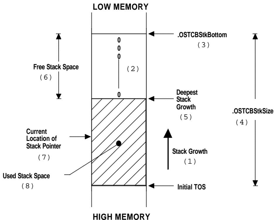
**Figure 4-2, Stack checking**
