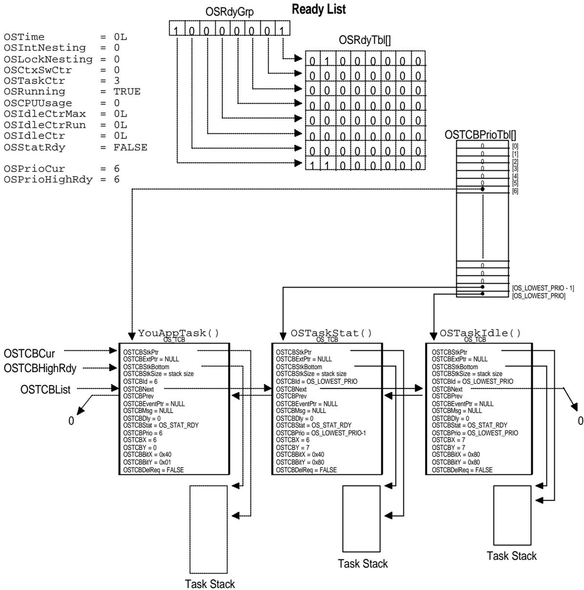
**Figure 3-9, Variables and Data Structures after calling OSStart()**
