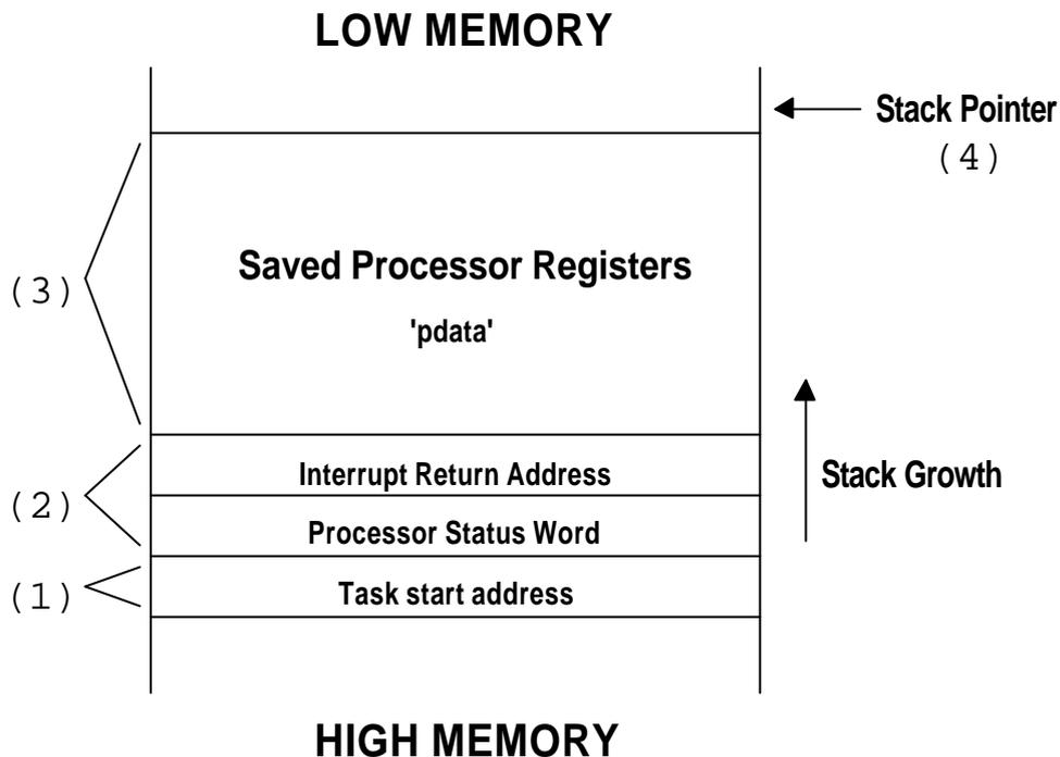
**Figure 8-4, Stack frame initialization with 'pdata' passed in register**
