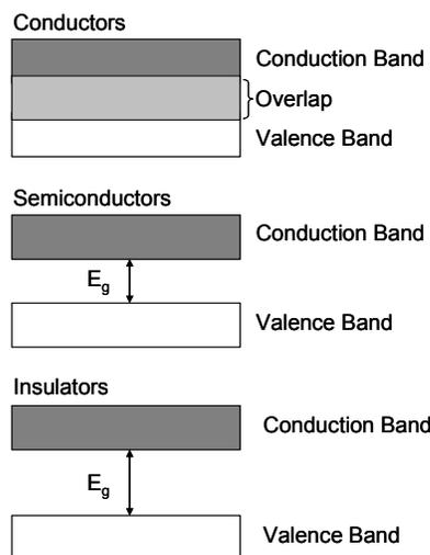
**Figure 1. Insulators, semiconductors, and conductors.** Band theory is used to explain the differences between conductors, semiconductors, and insulators which are chemically based on the differences in the amount of energy that it takes for the electrons in these materials to transfer from the valence band, the outermost shell in which electrons in a material travel, and the conductance band, where these electrons can freely move and be part of an electric current.
