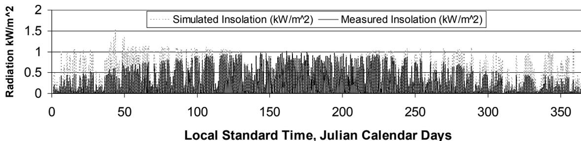
**Figure 5. Simulated and Raw Data Insolation.** *The model was used to calculate an hourly multiplication factor which was used to convert actual insolation data for a surface with a slope,  $\beta$ , of  $0^\circ$  to that for a surface with a slope of  $37.45^\circ$ . The raw insolation data was obtained from the Elora Research Station (Elora, ON) and was used to provide a basis for solar insolation for the city of Guelph, ON.*
