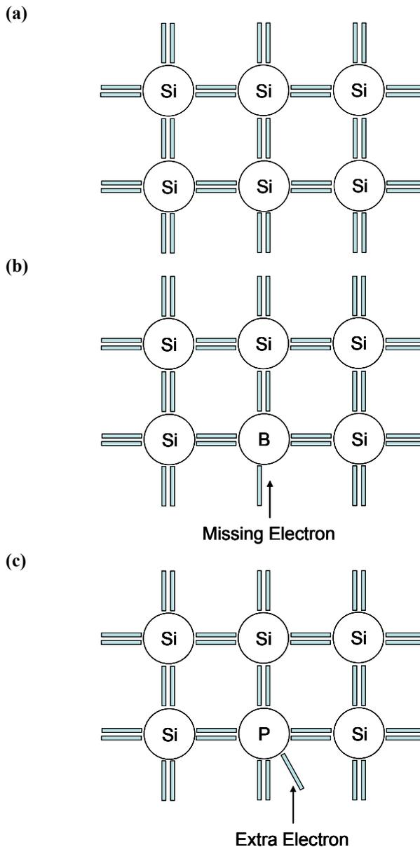
**Figure 2. Valence Electrons of Silicon and Doped Silicon.** *The valence electron, represented by the grey bars are indicative of the location of electrons shared between the atoms of silicon, phosphorous or boron. In (a) the location of the electrons in pure crystalline silicon is represented; in (b) the effect of the doping of silicon with boron is shown; in (c) the effect of doping silicon with phosphorous is shown.*
