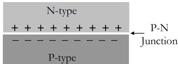
**Figure 3. The P-N Junction.** *The shift of charges across the interface of the P-N junction of silicon doped with boron (P-type) and phosphorous (N-type).*
