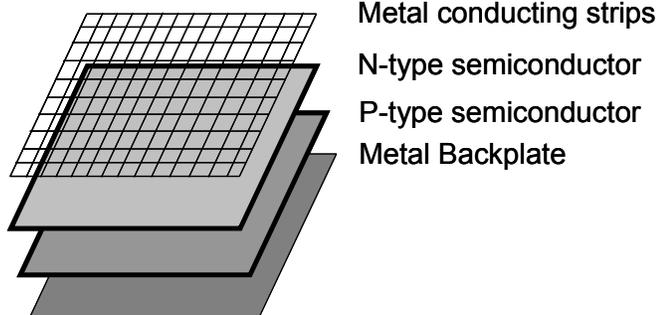
**Figure 4. PV Cell components.** *The cell primarily consists of four major components: the backplate, P-type semiconductor, N-type semiconductor, and conductive metal strips.*
