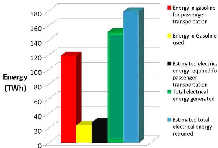
**Figure 3. Energy use in Ontario, 2006. Energy used in the form of gasoline is on the same order of magnitude as the total electrical energy generated. Data taken from IESO (2008).**
