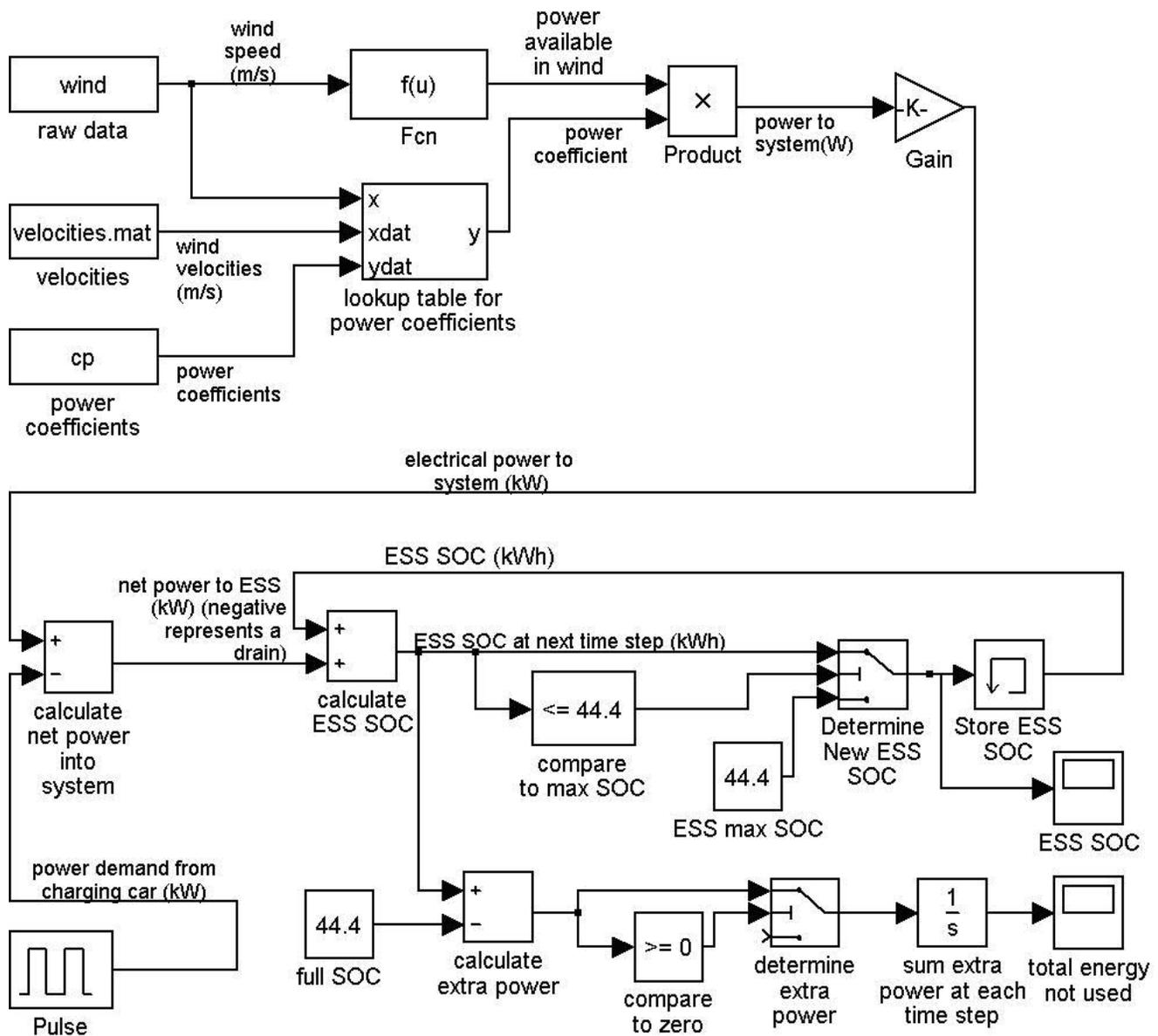
Figure 7. Simulink model used to simulate the wind/battery hybrid system. System parameters can be modified to predict changes in system performance, if required.
