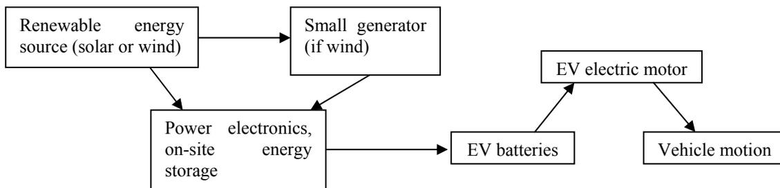
**Figure 2. Flow of energy from renewable source to charge a single EV from an off-grid system. Electrical power is generated by a small renewable power source. On-site power electronics and energy storage condition the power such that it can be used to charge the EV's battery.**
