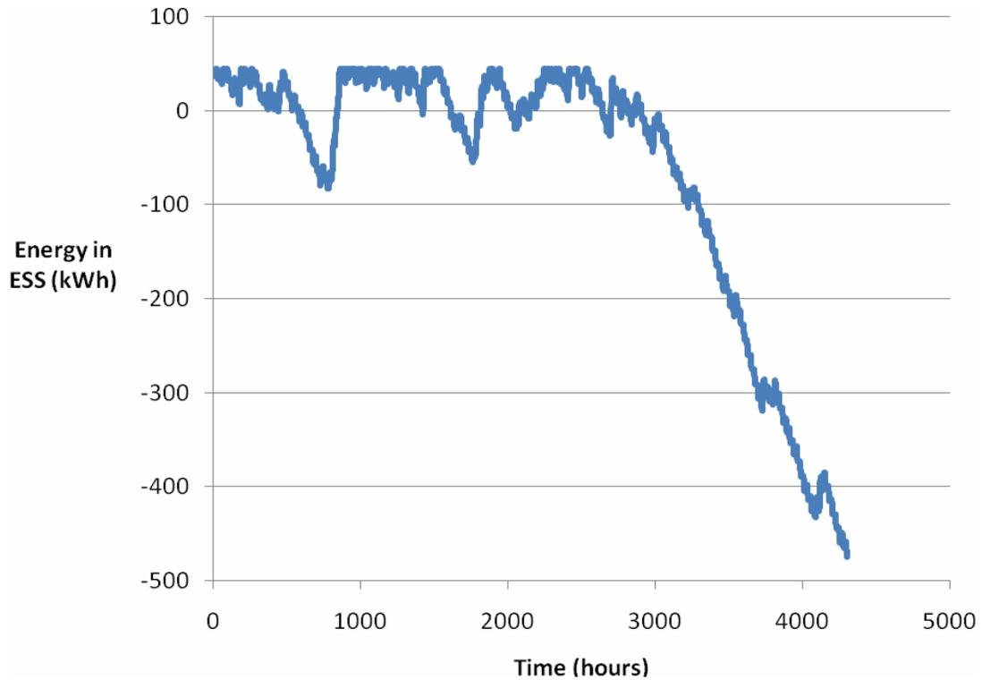
**Figure 8. Variation in the battery's state of charge as a function of time. SOC is on the y-axis, in kWh, while time is on the x-axis, in hours. Site is in Guelph, Ontario, with a battery capacity of 44.4 kWh.**
