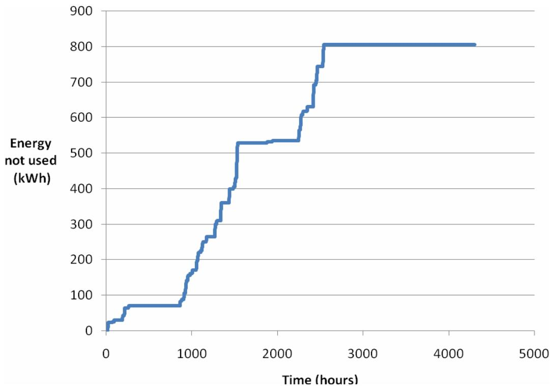
**Figure 9 – Excess energy in the wind as a function of time. Energy is on the y-axis in kWh, and time is on the x-axis in hours. This represents energy that could be extracted from the wind, but isn't, because both the car battery and on-site battery are already full.**
