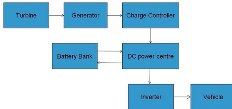
**Figure 6. Proposed configuration for an off-grid, wind/battery hybrid electric car charging system.**
