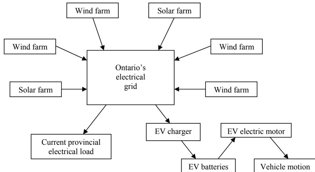
**Figure 1. Flow of energy from renewable sources to charge one or more EVs. Power is generated at distributed facilities and added to the grid. Electric cars charge their batteries from this increased renewable capacity. The energy is eventually converted into vehicular motion by an electric motor.**
