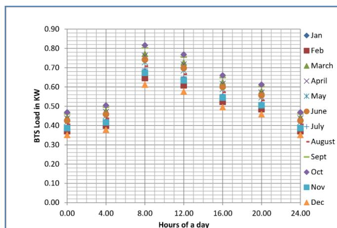
Figure 3: Load Pattern of BTS
