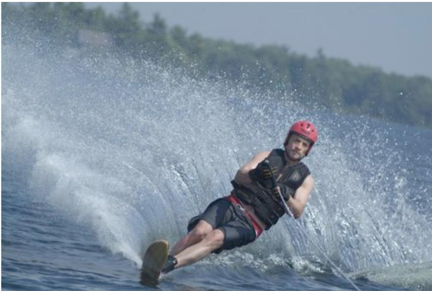
**Figure 2** – A test subject shown during a cutting maneuver while using a Maherajah Retro Fastback slalom ski and wearing the instrumented helmet. This subject reached a velocity of 124% of boat velocity, over 70 km per hr / 42 mph when cutting.
