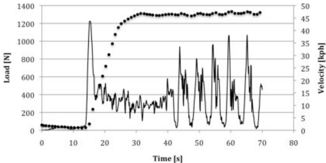
**Figure 3** – Typical data recorded for water starting, straight running and cutting on a Fastback slalom ski. Rope loads (continuous line) and boat velocity (dotted line) are shown.
